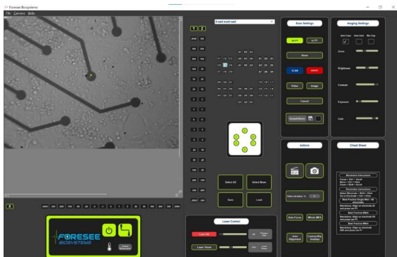
Figure 5: Software FB_Alps: a. Information card; b. Camera view; c. MEA layout and control buttons; d. Laser control; e. Scan settings; f. Image settings; g. Action panel; h. Cheat Sheet.
